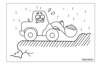
This machine is intended to be used only for excavation and loading. Do not use this for pulling up materials. Unlike a crane, this machine is not equipped with devices needed to pull up things.
