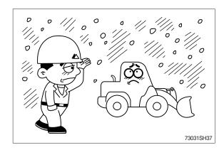
Put the chains on the tires when moving or working on the snowed and frozen road, and avoid doing sudden start, stop and swing.
